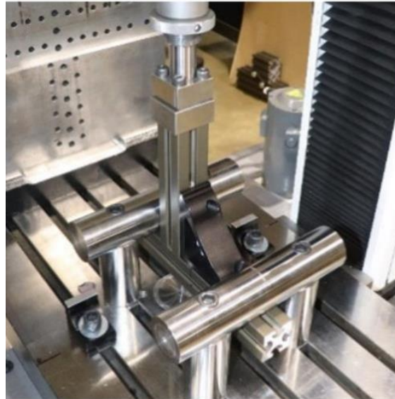
Figure 7: 40mm HD Corner Bracket mounted on 40x40 4-Slot HD Extrusion in Tension
