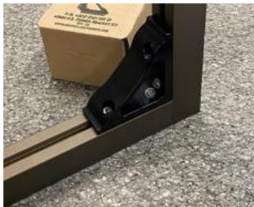
Figure 18: 40MM HD Corner Bracket - 40 x 40 2-Slots Profile Test Assembly
