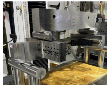
Figure 16: 40mm HD Corner Bracket Moment about Y-axis Orientation 1 (right) test setup
